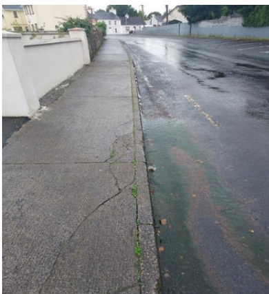
DYE TEST TO IDENTIFY SOURCE OF POLLUTION.
